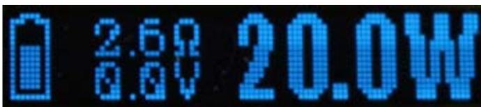
**Volts display (V):** The current or most recent output voltage being supplied to the atomizer.
